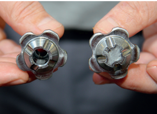
Blank formed components (right) are processed into finished parts (left) on the Mikron VX-10.
