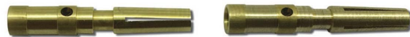
Examples of lead-free brass electrical connectors: on the left, machined with dedicated technology, on the right, machined with traditional technology
