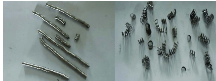
Examples of lead- and sulfur-free steel chips. Left, with dedicated technology; right, with conventional tools.
