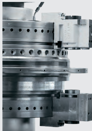
adjustable work station supports (above and below) with embedded indexing table.
