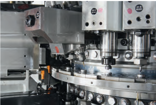
Machining units operating from all directions
