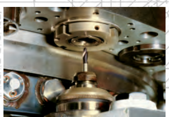
Drilling from below
