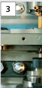
Pre turning on top, drilling from below
