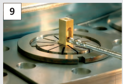
9 Sideways drilling and thread cutting
