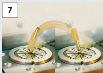
Part turn-over in different section collet
