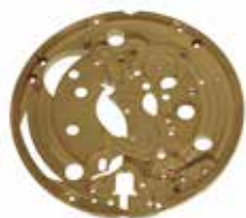
Watch Plate Brass, on Mikron NRG
