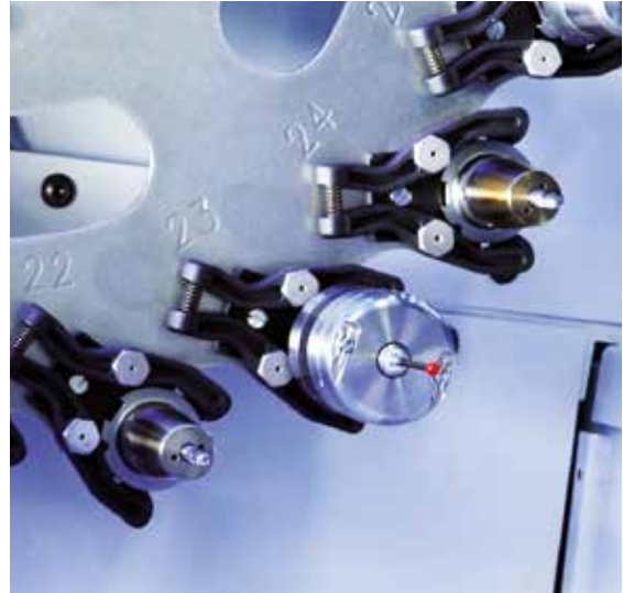
The measuring sensor can be loaded in just 1 second like any other work tool.
